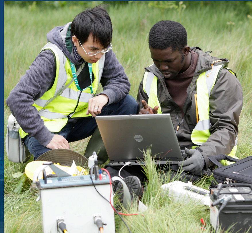
MSc Petroleum Geophysics students acquire seismic data at Humbly Grove (2011)
